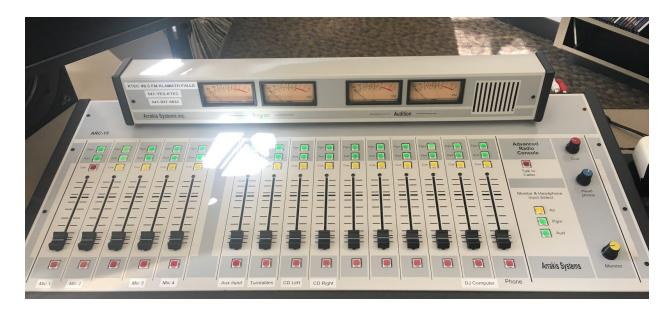
Each channel contains an on/off switch and volume fader. The microphone channels contain talk button, Audition (AUD) button, and Program (PRGM) button. The audio source channels contain Cue button, Audition (AUD) button, and Program (PRGM) button.
